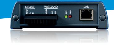
The Wiegand Interface Module ensures an easy integration of the ANPR Access (HD) into any existing or new access control panel that support Wiegand. This module converts license plate numbers that are captured by the ANPR Access (HD) into Wiegand ID strings.
